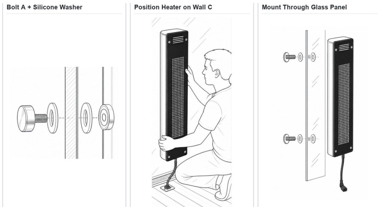
Figure 14. Full-spectrum heater bolted through the Glass Wall (C), silicone washer on every bolt.
