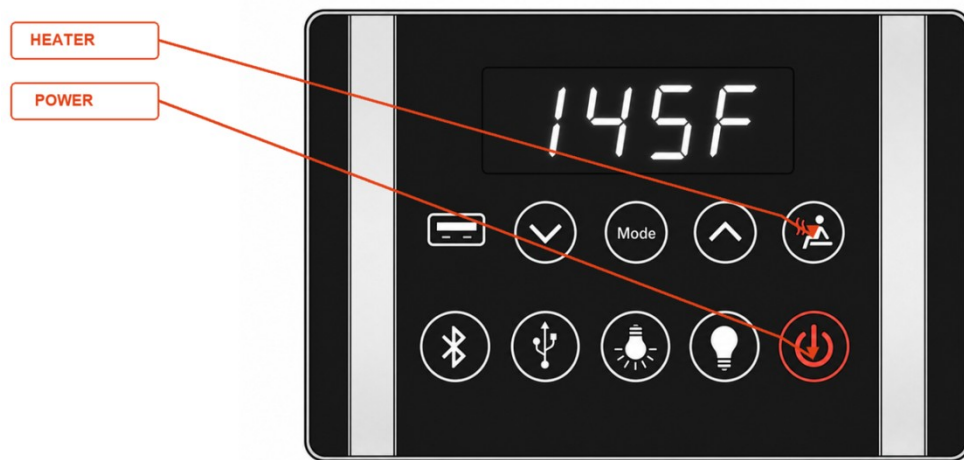
Figure 21. Main control panel.
