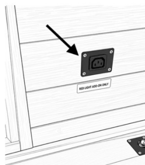
Figure 25. Red Light Therapy Panel: verify washers, mount through the door glass, connect power beside the door.
