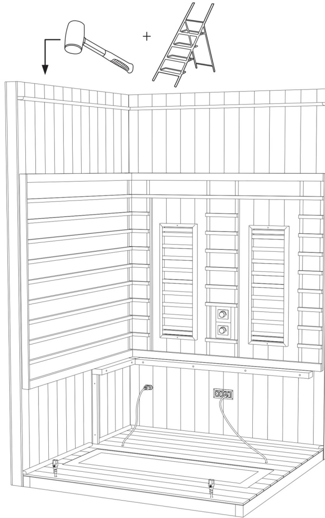
Figure 6. Left Panel (A) buckled to the Back Panel (B) and tapped down with the rubber mallet from the ladder.
