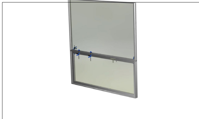
Fig 14. Once both the strong and opposite sides of the jamb have been fully joined, we recommend keeping a clamp at the top, bottom and middle of both the strong and opposite side until the silicone cures.
