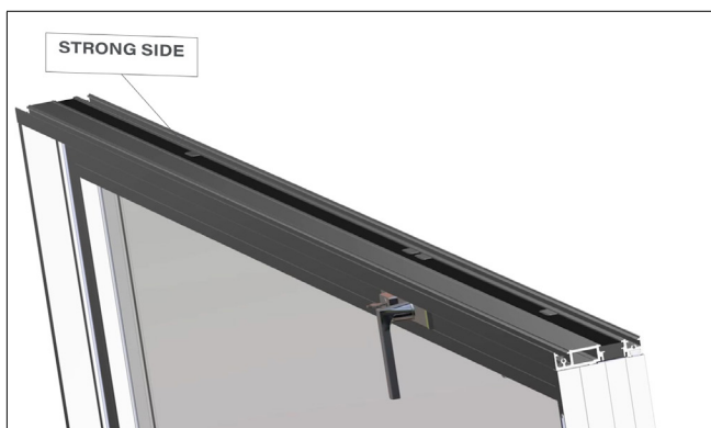
Fig 1. Begin by locating the side where you wish to mull together with another door or window.
