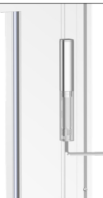
Fig 8. Use an Allen wrench to access the threaded adjustment nut inside.
