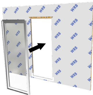
Fig 7. Next, install the Door Assembly. With assistance, tilt the unit into the rough opening. Use shims as needed for a snug fit.
