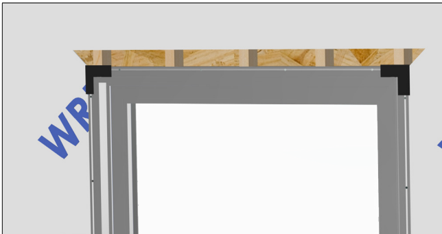
Fig 9. Cover all corners with corner gaskets, ensuring full coverage of the nail fins.
