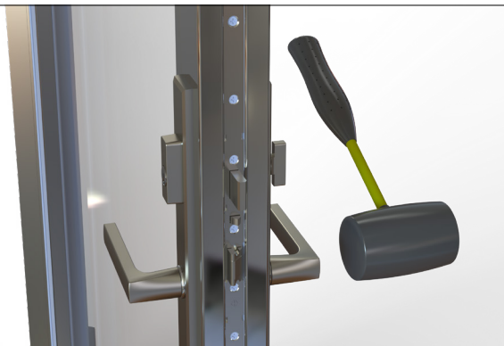
Fig 3. Once the handles are in place, use a Mallet to tab the Handles into place. Make sure the Handles are fully in place, but do not over tighten.
