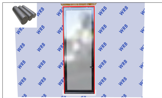
Fig 14. Finally, Seal the Exterior. Apply backer rod and sealant around the perimeter—vertical sides and head jamb—according to standard procedures.
