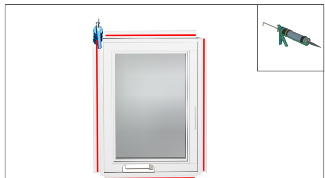
Fig 4. After pre-drilling, apply sealant along the interior of all 4 nailfins.
