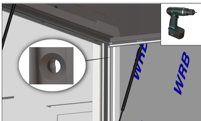
Fig 9. Use a drill, to countersink and drill all anchoring holes through the interior frames.
