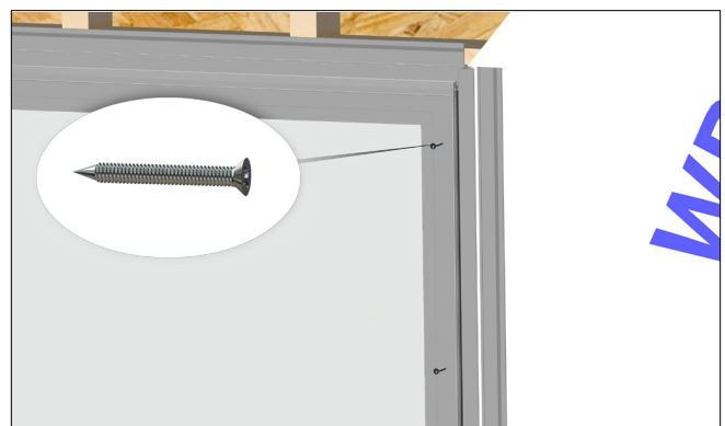
Fig 8. Secure all Nail Fins to the structure using #8 x 1 1/4" self-tapping screws.
