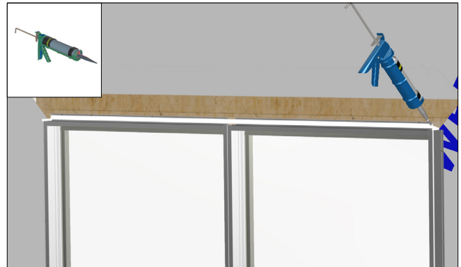
Fig 6. Next, lay a steady bead of sealant along the entire length of all nailfins on the head.
